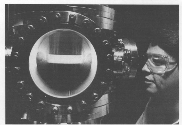
PEERING through "portholes" in the GEC RF (radio frequency) Reference Cell is Ben Aragon (contractor). Sandia initiated and led a national effort to develop the standard plasma research reactor, which is already benefiting US research in plasma etching, an essential step in modern microelectronics manufacturing. (GEC stands for Gaseous Electronics Conference, where the Reference Cell concept was first discussed in 1988.)
